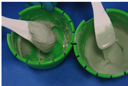
The difference in the viscosity is clearly apparent immediately after the mixing: High-viscosity bone cement (left), low-viscosity bone cement (right).
