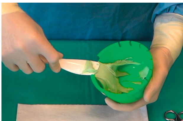
Optical test: Homogeneous cement dough shows no powder nests
